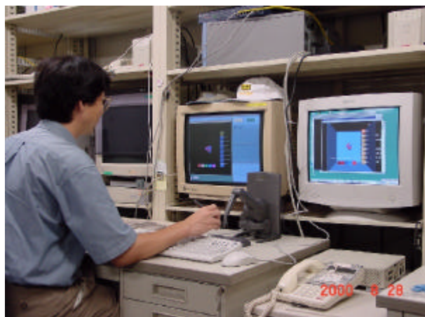
Fig. 6 Illustration of the scanning of a molecule using the PHANToM™
